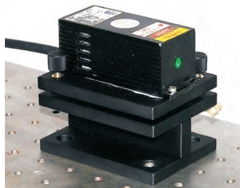
Fig. DPSS Laser with Kinematic mount
